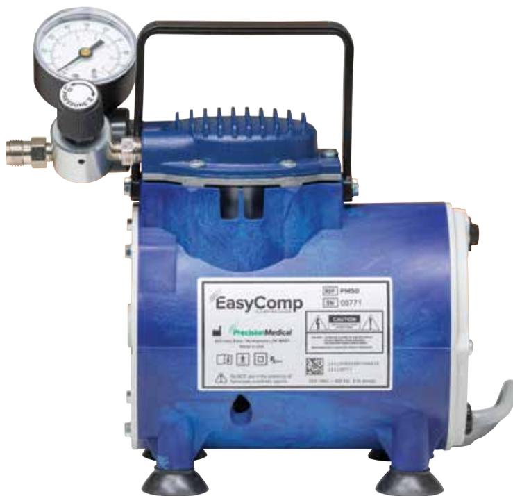
EasyComp Compressor is a lightweight, portable medical air compressor that delivers a minimum of 13 l/min of air flow at 50 psi. Weighing only 9.7 lbs, the compact unit has atop facing handle for additional ease. The built-in safety system protects the unit from overheating during operation. Soft, pliable suction cup feet secure the EasyComp to a flat surface and help reduce vibration.
